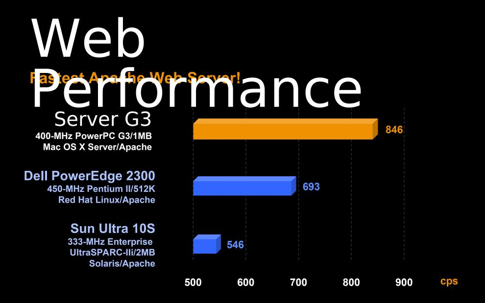
WebBench static HTML throughput with 60 PC clients in connections per second (cps) on 100BASE-T Ethernet. Results compiled by ZD Testing Analysis Group (www.zdnet.com/zdtag/reports/reports.html/).
